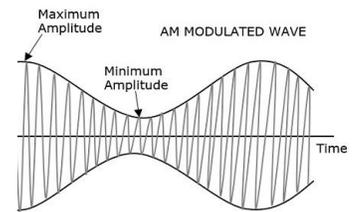
Amplitude modulation produces two new frequencies. The sum and difference of the carrier and base band frequencies. 14.253MHz and 14.247 MHz. in this example. These are the "side band" frequencies. The sidebands are mirror images of each other. Each have the same 3000 Hz information. There are four frequencies at the output of an amplitude modulator, the base band, the carrier, and two side bands. In other words, 3000 Hz, 14.250 MHz, 14.253MHz & 14.247MHz.
