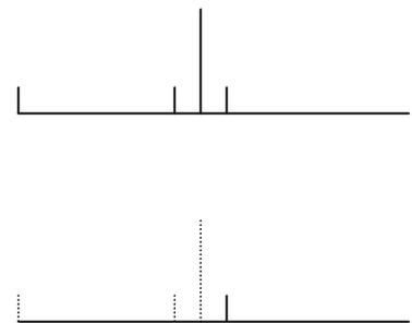
Fig. 4 represents those four frequencies as they would appear on a spectrum analyzer. The tallest line is the carrier. The lines on either side of the carrier are the upper and lower sidebands. The line at the left is the 3000Hz base band.
